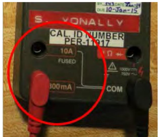
I will tell you that on this particular meter it really doesn't change the reading, as all of you pointed out to me in the first boo-boo above. But, for safety sake, it is important that you have the connections to the meter correct as well. This is so you are operating everything in a fused circuit, and not just hanging it out there where you could potentially burn up the meter, or worse, YOU.
