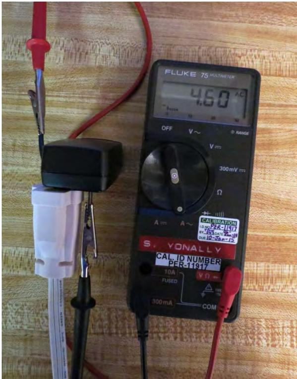
In order to know just how much each one of these little creatures are costing me, we need to measure them for power utilization when nothing is plugged into them and they are still plugged into the wall. So, with a little experimentation and remembering Ohm's Law, we know that Volts x Amps = Watts, and Watts are what we care about. Your power company charges you for kilowatt-hours. (One thousand watts for one hour is a kWh).
